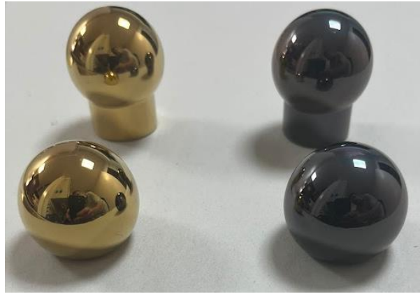
Fig. 2. Femoral heads coated with thin layers of TiN and TiO 2 with a thickness of 1.5 μm deposited by DC sputtering.
