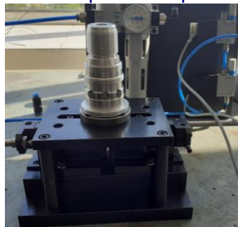
Figure 3. Inner diameter measurement system
