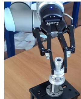
Figure 4. UR10 manipulator robot with 2F-140 adaptive gripper
